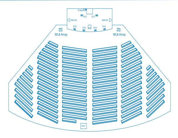
At this point, we assume the congregation is moving into a purpose-built facility and the entire Stage 4 system can move in with them. Here's where the scalability of the WideLine-8 system becomes apparent. Up to eight extra WL3082 line array loudspeakers can be added without the need to purchase any additional amplifiers.
