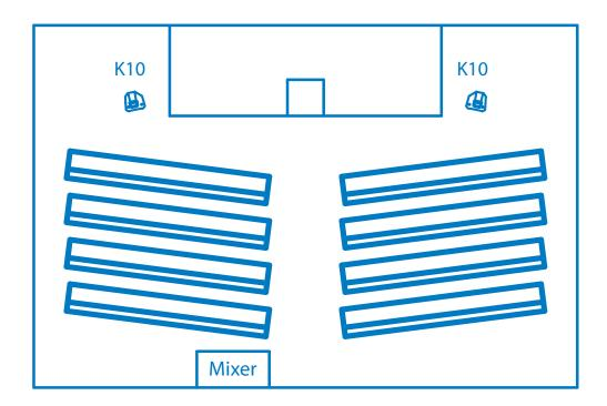
This basic system is intended to provide sound reinforcement for speech, vocals and acoustic music. It is extremely simple to transport, set up and operate – even for novice volunteers. It will provide the coverage and acoustic output for a small rented space such as a storefront or community hall.
